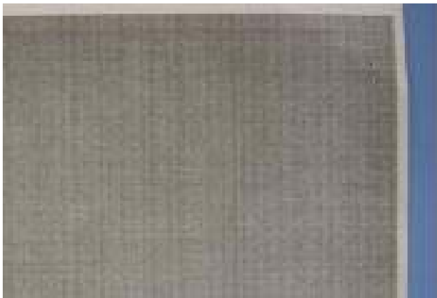
Sample 5 (Uneven image density caused by toner filming on the development roller)
