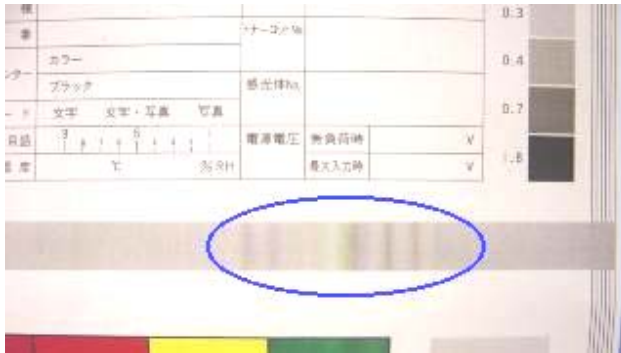
Sample 2 (Uneven image density caused by scratch on the OPC belt)
