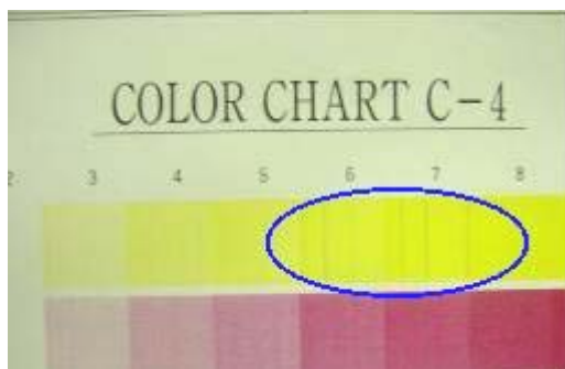
Sample 3 (Uneven image density caused by insufficient cleaning of the OPC belt)
